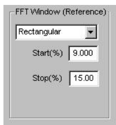
Selecting a Rectangular Force Window and Setting Points for 9% and 15% Selected and set in the FFT Setup Tab.
